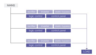
ABB's modular DPA UPScale ST is built of self-contained modules that include the entire UPS hardware and software; hence, it eliminates all the common parts which are potential single points of failure.
